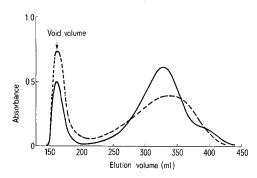
Gel filtration pattern of 100 mg of fraction  $\rm E_2$  on a Bio-Gel A-1.5 m column (2.5  $\times$  80 cm), equilibrated with 0.05 M ammonium acetate buffer, pH 7. Flow rate 25 ml/h. ——, Absorbance of the eluent monitored at 254 nm with an L.K.B. Uvicord I; -----, Folin-Lowry colour at 750 nm. Activity eluted between 150 and 180 ml.
